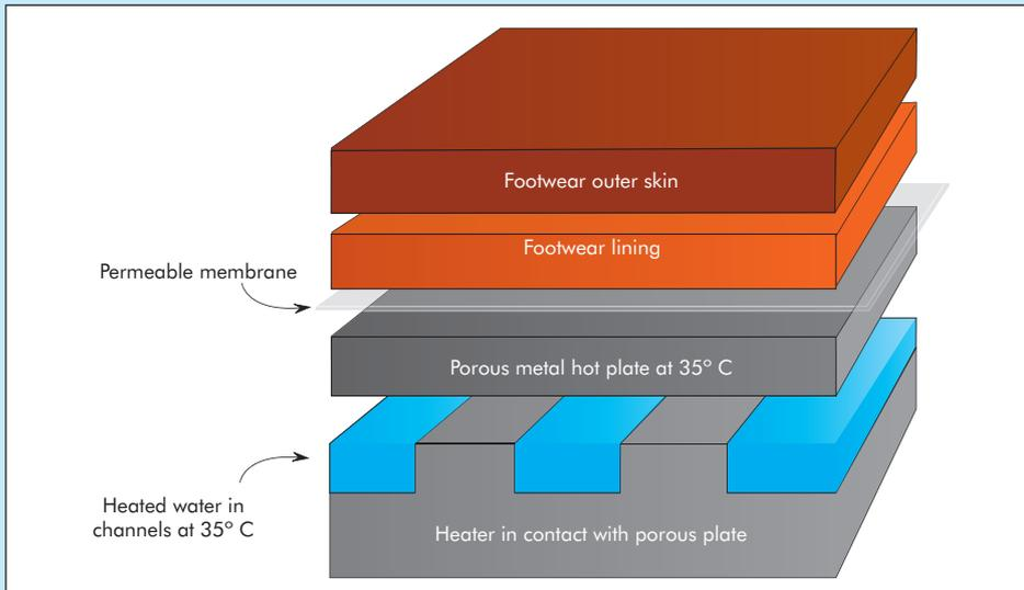
Figure 3: The principles, left, and operation, right, of a guarded hotplate
