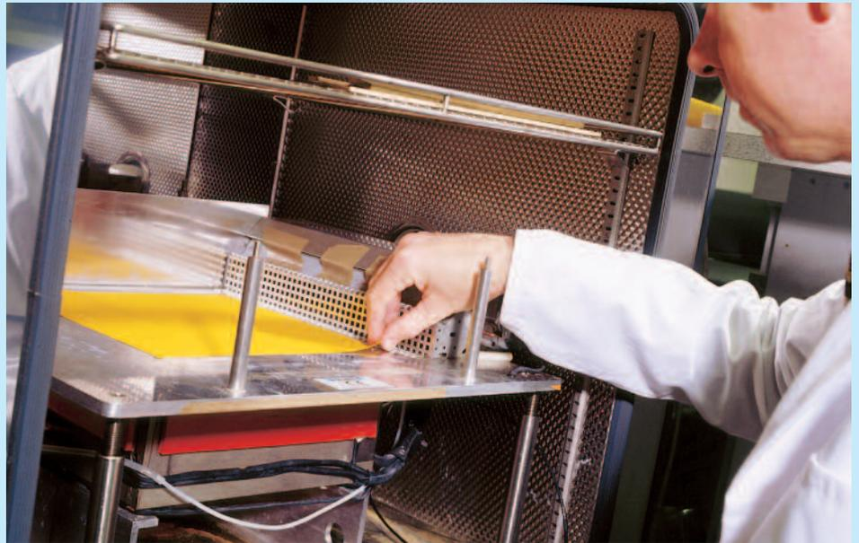
Figure 1: Placing a specimen on the hotplate prior to testing
