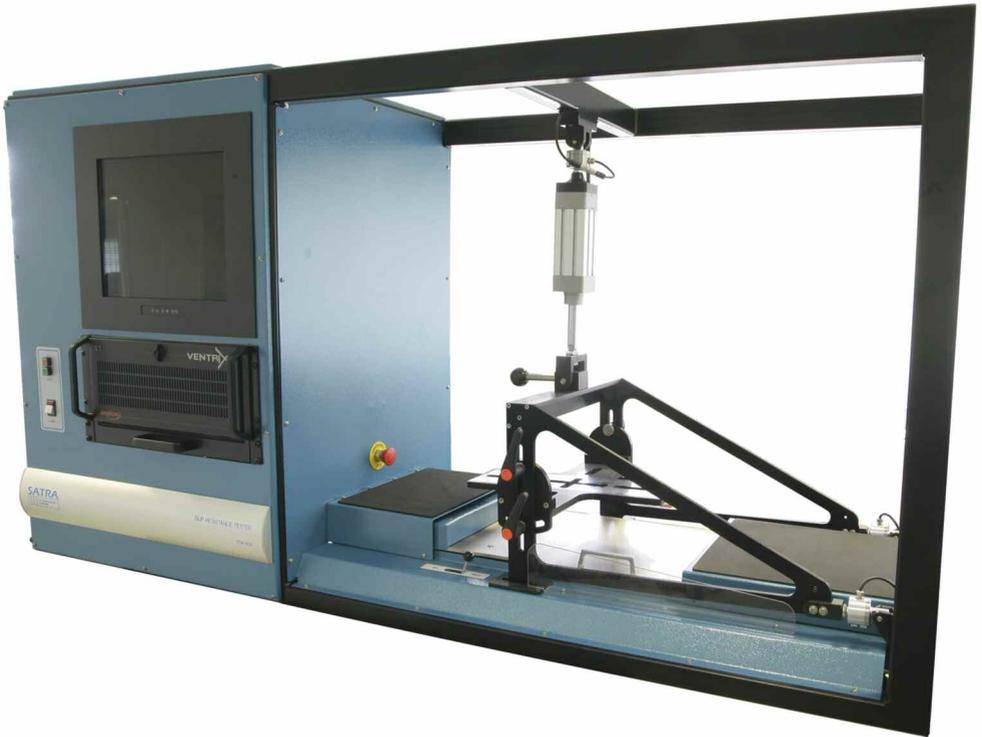
**STM 603** can test a wide range of footwear on various surfaces and simulated conditions, for example dry and wet tile, or frosted and smooth ice. Footwear, surfaces and test conditions can be easily set up. The machine incorporates a specially-designed control and data acquisition system which provides the user with the coefficient of friction for each test sample, as well as providing graphical representation of the test data.
