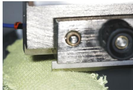
Figure 1: The STM 610 blade cut tester consists of a straight blade which is drawn across the sample mounted on a curved surface
